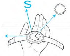
Figure 1. Using a Wristwatch to Find South.
